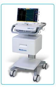
assessed by comparing observed muscle responses with the expected maximum contractions. The system includes an electrical pulse generator, appropriate electrodes, sensors to detect muscle response, and audible and or visual indicators to track and notify the surgeon in real time of nerve condition visually and audibly.
